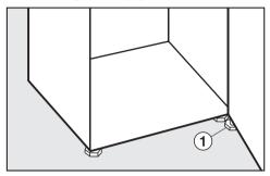
■ Ensure that you unscrew adjusting foot ① until it sits on the floor. Then unscrew the foot by a further 90°.
